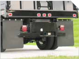
COMBINATION CLASS V HITCH AND ICC BUMPER
