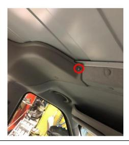
B. Taking off the headliner will reveal the below OEM brackets. Place the frame kit in the vehicle and align it such that the backing plates (CRF 28-1100-006) are centered between the two OEM brackets. Then adjust the frame kit so that it sits evenly between the Curbside and Roadside. Mark (2) hole locations on each side, using the backing plate pre-drilled holes as a template.
