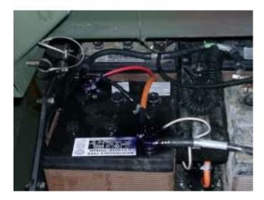
13. Secure wires to factory harness with wire ties.
