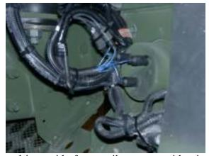
10. Route power harness down frame to battery box along drivers side frame rail – secure with wire ties.
