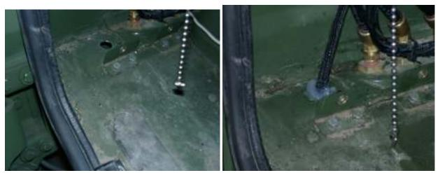
15. Mount control module to backside of grill, above openings, wire tie in place.
