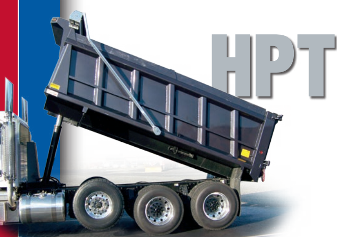
DuraClass HPT features fully enclosed front corner posts.
