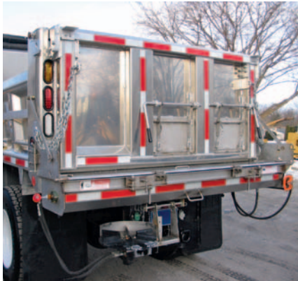
Tailgate bracing incorporates a 6-panel design standard. Or choose, as shown, to add up to 3 patchgates for additional versatility.
