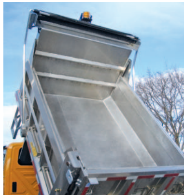
A 6" one-piece, bevel plate, floor-to-side bracing increases material flow. Two front horizontal V braces provide additional rigidity.
