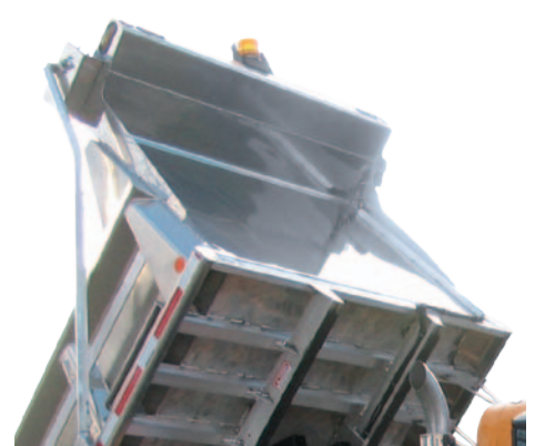
The aluminum design features a stacked understructure of 5 3/4" I-beam longmembers and 4" crossmembers on 12" centers for maximum floor support.
