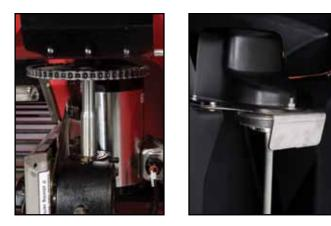
**DUAL ELECTRIC MOTORS** power the conveyor and spinner, giving you independent control of material delivery and spinner speed. Electric motors mean low maintenance and reliable starting.
