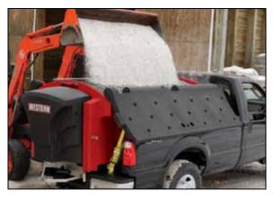
**OPEN POLY HOPPER COVERS** protect the truck bed from material overflow during loading.
