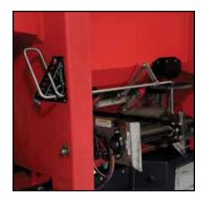
**ADJUSTABLE FEED GATE** regulates material flow to your exact requirements.
