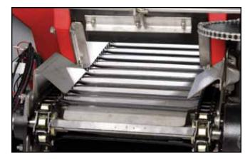
STEEL PINTLE CHAIN CONVEYOR and corrosionresistant stainless steel housing provide strength, reliability, and consistent material flow.
