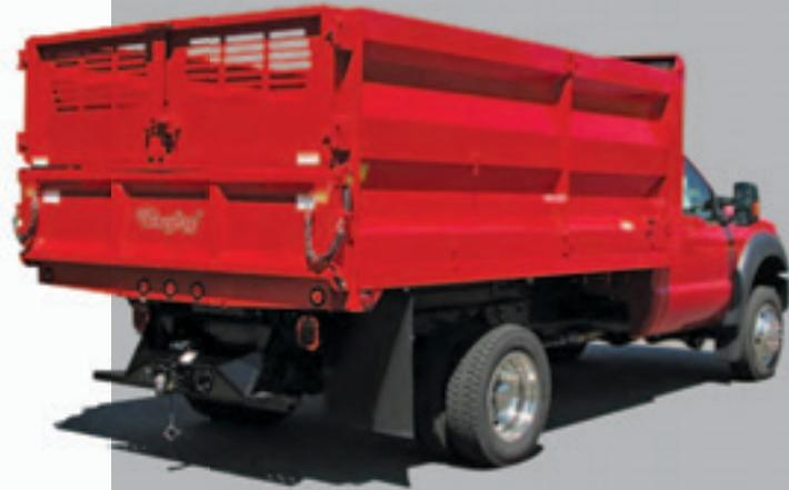
Rugby's Landscape Uni-Body features 48" tall stakeless sides with a centered horizontal formed rib and a 2-piece smooth steel floor, with a center seam welded underneath. The body features 10 gauge construction throughout and is available with either the traditional 2-piece barn doors over a drop down tailgate or with a 2-piece full height, double rear swing out doors. Available 12' and 14' lengths.
