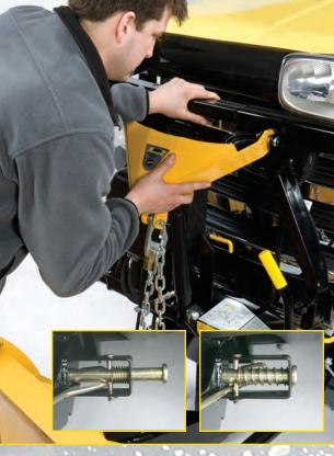
With just a little push on the headgear, the spring loaded pins pop into place, completing the attachment of the Minute Mount® 2 System.
