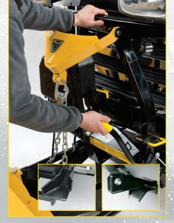
To attach the snowplow, simply drive into the mount. The attachment arms and lower gear are flared both vertically and horizontally to make the drive-in connection easy. Once the mount has completely engaged the lower gear, raise the pin release handle, readying the spring loaded connecting pins for engagement.
