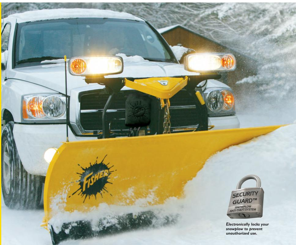
With the increasing popularity of smaller and lighter four-wheel-drive vehicles in mind, Fisher Engineering has designed a snowplow that is compatible with the reduced axle capacity of these vehicles while meeting the needs of the personal use snow plower.
