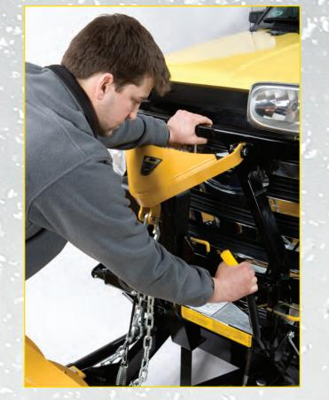
Removing the snowplow is even easier. After lowering the blade, pull out on the jack lock and the jack automatically drops to the ground. While pushing on the headgear, lower the pin release handle to disengage the connecting pins. Unplug the electrical connectors and you are done!
