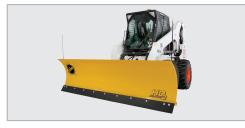
The HD2 plow is also available for skid-steers with a universal skid-steer mounting plate for fast and easy hook-up.
