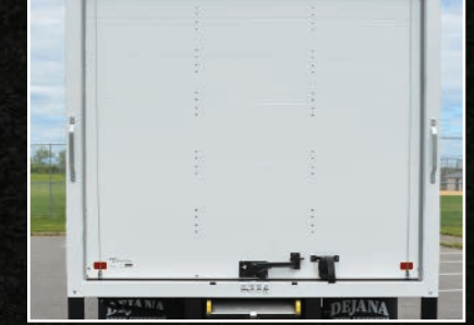
• Extreme duty composite roll-up rear door stainless steel/ alum. Hardware 1" diameter HD roller hinges • (2) Assist handles
