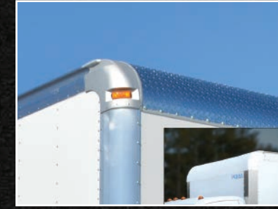
• 10" front radius to protect from branches and debris. Diamondplate (DRW); Fiberglass (SRW) • 5" radius aluminum corner castings
