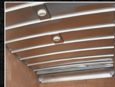
• Anti snag roof bows • .032 Aluminum roof • No exposed wiring
