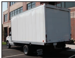
4" Structural Long Sills 3" Cross Member Height Whiting Roll Up Doors Recessed Running Lights
