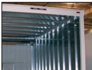
Anti Snag Roof Bows .032 Aluminum Roof No Exposed Wiring
