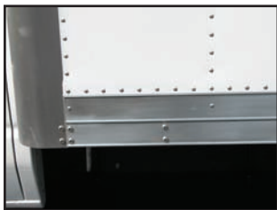
2" Spacing on Seams, 4" on Ribs Radiused Cornerposts Aluminum Top & Bottom Extrusions
