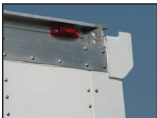
Integral Roof Rain Gutter System directs rain away from back door (Standard on Pro Models)
