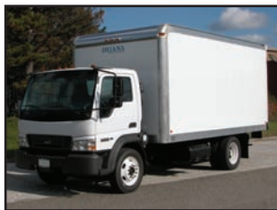
.040 Pre-Painted Aluminum Aluminum Treadplate Radius Extruded Aluminum Corners
