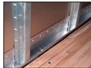
Galvanized "Z" Posts on 16" Rollup door with 2" rollers for smoother operation Beefy 4" x 5.6" rear post
