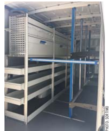
On the street side, the van provides storage for long components and tools, while curbside the driver has access to Flexx Rack shelving that can fold away if more space is needed.
