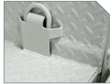
CARGO TIE-DOWNS (Pictured in steel. In-floor swivel D-rings available in aluminum.)
