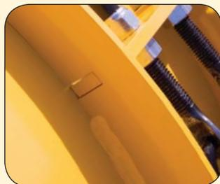
Slot and tab construction and laser cut ribs improve strength and durability. Robotically welded components make for high strength connections.
