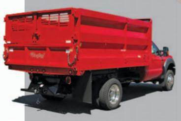
Rugby's Landscape Uni-Body features 48" tall stakeless sides with a centered horizontal formed rib and a 2-piece smooth steel floor, with a center seam welded underneath. The body features 10 gauge construction throughout and is available with either the traditional 2-piece barn doors over a drop down tailgate or with a 2-piece full height, double rear swing out doors. Available 12' and 14' lengths.
