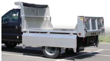
Fold down aluminum sides are lightweight and easy to operate.
