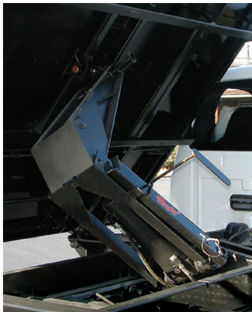
Multi-Directional dumping hoist specifically designed for MD Eliminator body.
