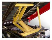
Automatic body bracing positioning
